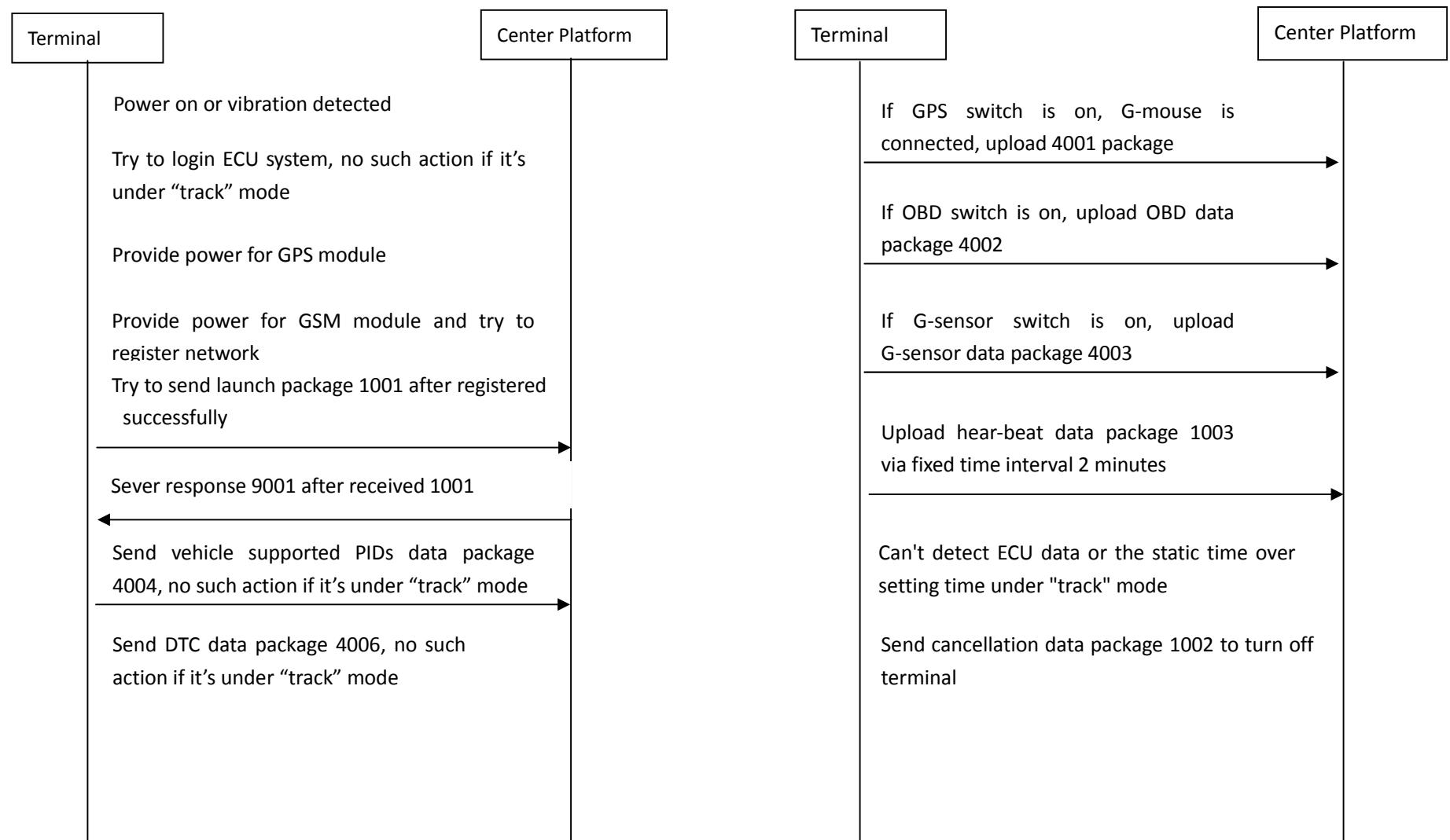
Send snapshot& freeze frame data package 4005, no such action if it's under "track" mode
